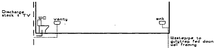
FIRST FLOOR PLUMBING SCHEMATIC 1 : 100
